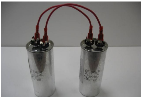
Two 40 uF capacitors wired in parallel.
