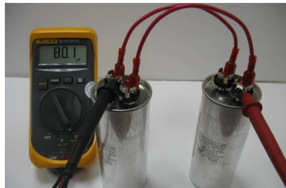
The total capacitance is 80.1 uF.
