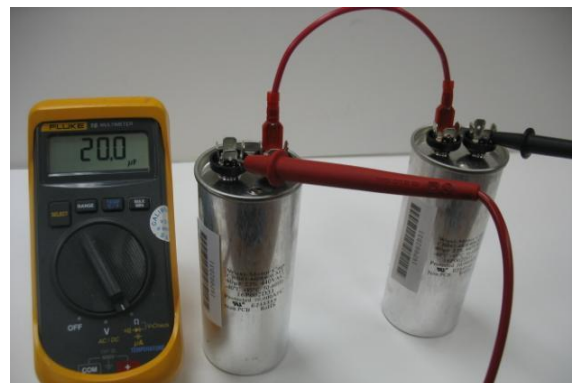
The total capacitance is 20 uF.
