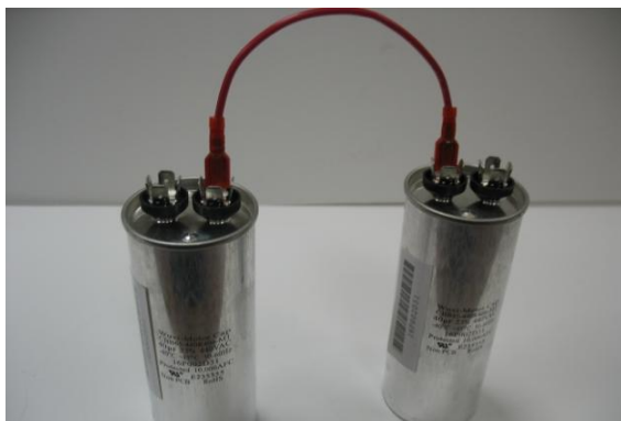
Two 40 uF capacitors wired in series.
