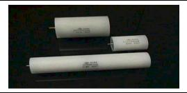
Type CH84 Capacitors offer superior electrical characteristics coupled with small size. Type CH84 Capacitors are wound with a compound film dielectric between sheets of Aluminum Foil. They are impregnated; silicon rubber filled, and sealed in a tough plastic case. Type CH84 Capacitors are designed for wide range of uses including power supply filtering, voltage multipliers, bypass, coupling, and suppression.
